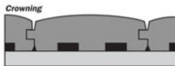
**CROWNING:** “Crowning” is the opposite of cupping: The middle of the board is higher than the edges of the board. This can occur when the surface of the floor encounters moisture. More often, it results when a floor has been sanded too soon after it has cupped. When this happens, the top edges of the board are sanded off, and thus are lower than the rest of the board when it returns to a normal moisture content.
